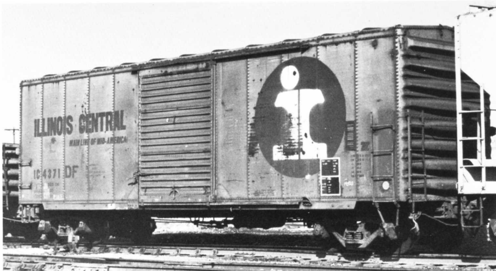
IC 4371 BOXCAR 40FT. PHOTO BY DAVID HUYCK. The 4000-4899 series cars were built by IC Centralia, IL car shop in 1957 and upgraded by IC. Cars equipped with DF load devices. Most of these were assigned to appliance loading in Herrin, IL and Evansville, IND. A few were assigned to Effingham, IL for air conditioner loading.
