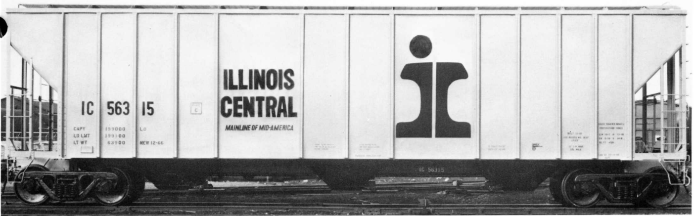
IC 56315 COVERED HOPPER. PHOTO BY ICRR - ICHS COLLECTION. The 56300-56799 series of covered hoppers were built by G.A.T.X. in 1966 & 1967 at E. Chicago, IN. The cars are 100 ton capy with 4700 cu ft capy. The cars are equipped with a 3 piece 44 ft hatch. These cars are assigned mainly to grain service.
