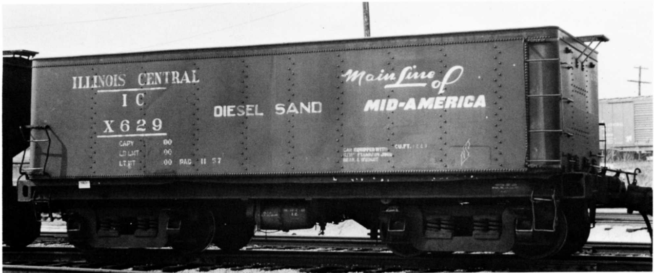
IC X629 SAND CAR. PHOTO BY BRUCE MEYER. Former IC water car. These cars were built by the IC and rebuilt by the Paducah, KY locomotive shop for diesel sand service, diesel fuel service or a combination of both.
