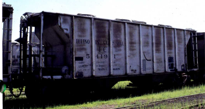
IC 54191. COVERED HOPPER. 54150-54299. ACF 1960. 70 ton capacity.
