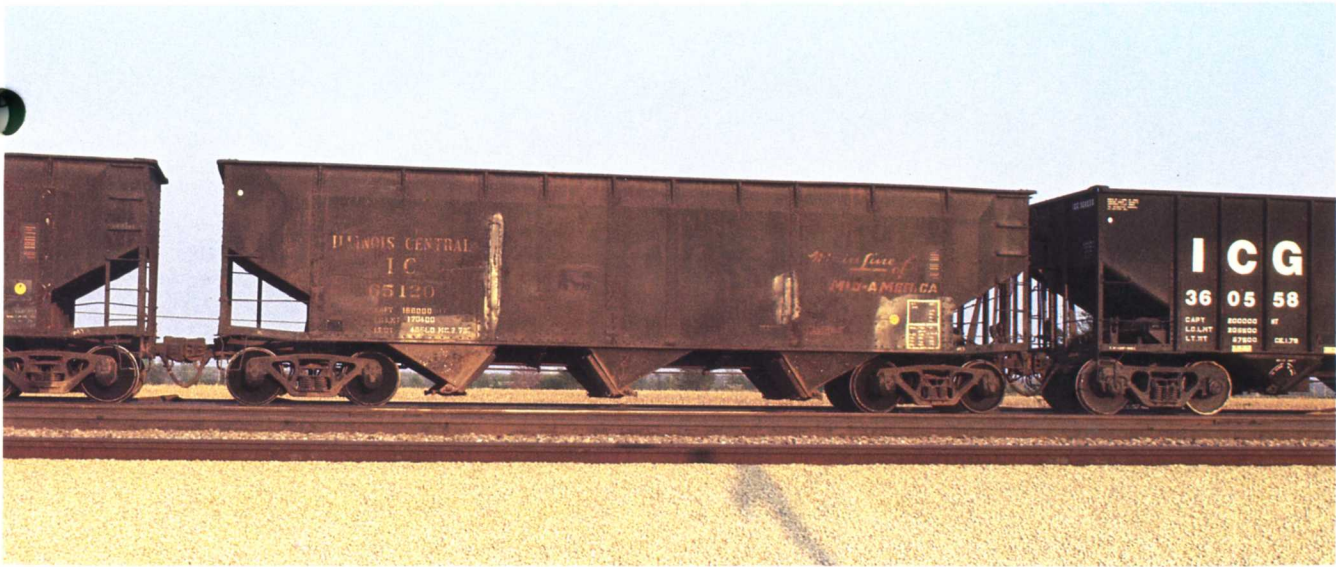
IC 65120. HOPPER. 65000-67999. ICRR 1964. 70 ton capacity.
