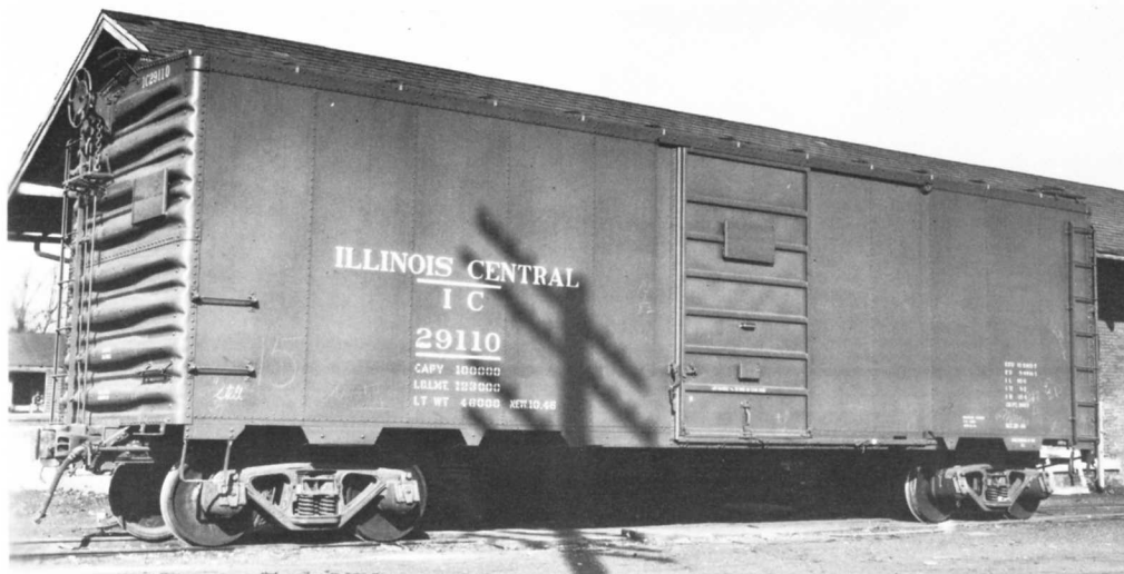
IC 29110 BOXCAR 40FT. PHOTO BY M.D. McCARTER. The 29000-29499 series cars were built by the IC Centralia, IL car shop in 1946.
