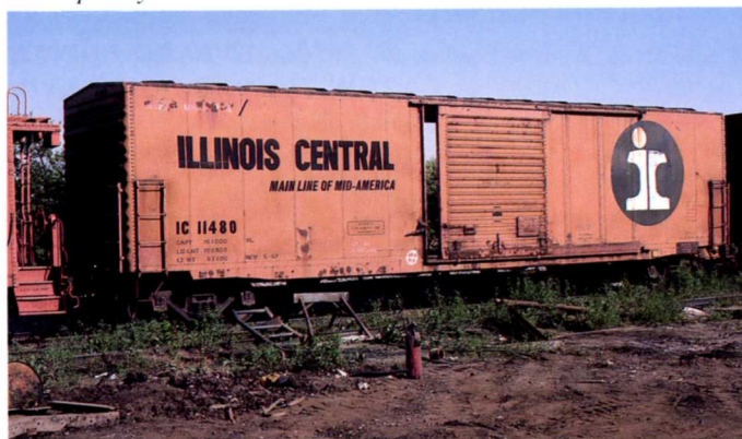
IC 11480. 50FT BOXCAR. 11300-11499. ACF 1967. 70 ton capacity.
