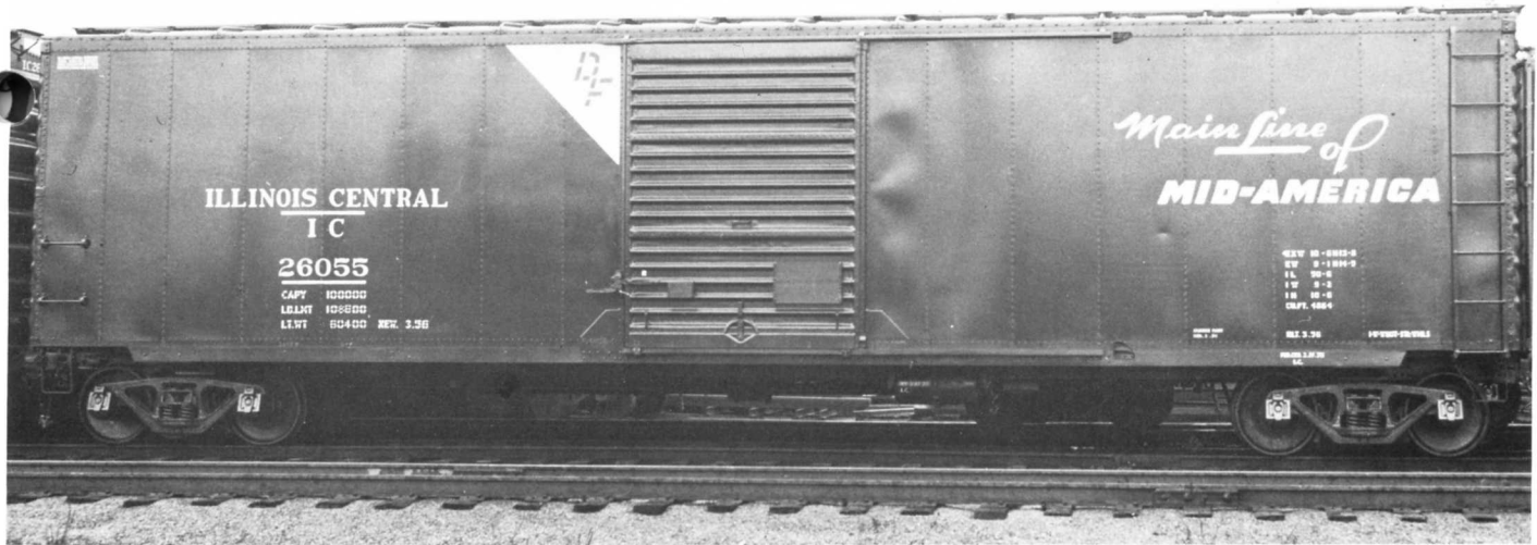
IC 26055 BOXCAR 50FT. PHOTO BY ICRR - ICHS COLLECTION. The 26000 - 26099 series cars were built by the IC Centralia, IL car shop in 1956. The cars were equipped with 9 belt DF loading devices and 1 1/4" wood floor decking.
