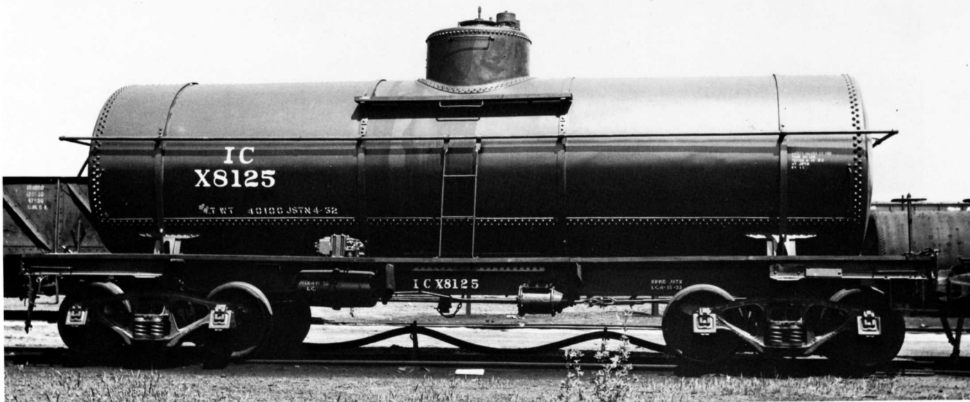
IC X8125 TANK CAR. PHOTO BY G.V. CARSON - ICHS COLLECTION. The X8125-X8129 series tank cars were built by ACF in 1905 for the IC and originally numbered 1-5.
