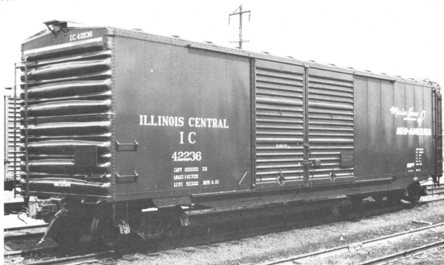
IC 42236 BOXCAR 50FT. PHOTO BY ICRR - ICHS COLLECTION. The 41800-42549 series cars were built by the IC Centralia, IL car shop in 1961. The cars were equipped with 2 1 / 4 " wood flooring and assigned to auto parts service.
