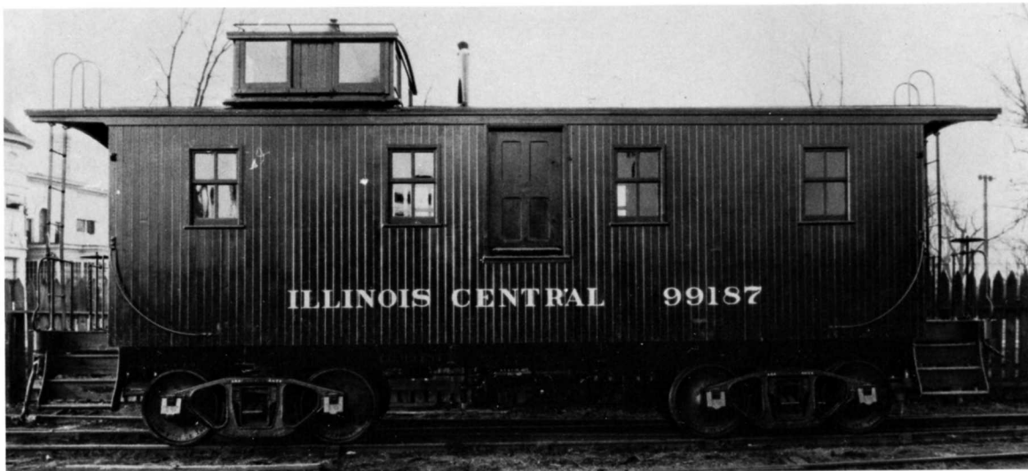
IC 99187 WOOD CABOOSE. PHOTO BY ACF - IC HS COLLECTION. The 99181-99200 series cabooses were built by ACF in 1923. They were later renumbered by the IC to 9181-9200.
