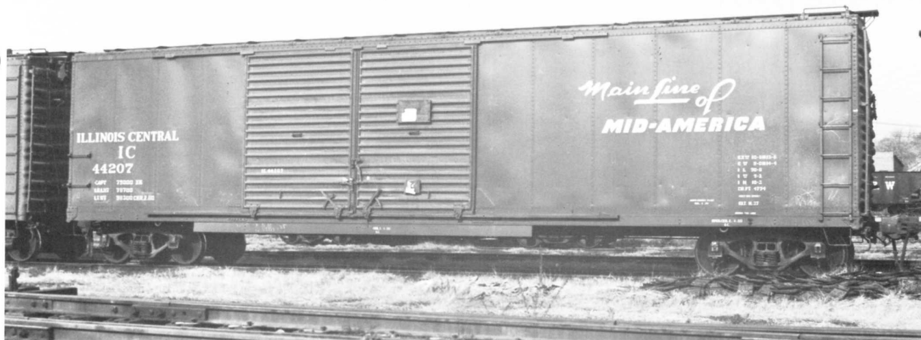
IC 44207 BOXCAR. PHOTO BY JAY WILLIAMS. The 44000-44281 series cars were built by G.A.T. in 1937 as 161501-161700 series cars. They were rebuilt in 1950 by the IC Centralia, IL car shop and renumbered into the 44000 series.
