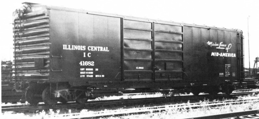
IC 41682 BOXCAR 50FT. PHOTO BY ICRR - DAVID J. DAISY COLLECTION. The 41600-41799 series cars were built by the IC Centralia, IL car shop in 1959. Equipped with DF load devices.
