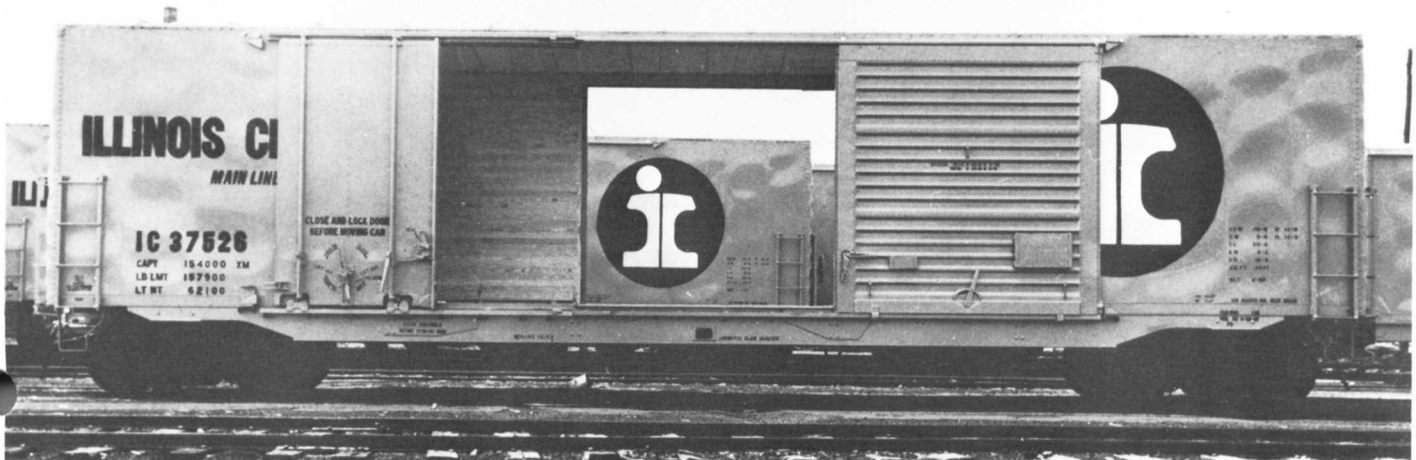
IC 37526 BOXCAR 50FT. PHOTO ICRR - ICHS COLLECTION. This car is part of the 37500-37699 series built by Pullman Standard in 1967 and equipped with combination doors and 2 3 / 8 " Durawood floor decking.
