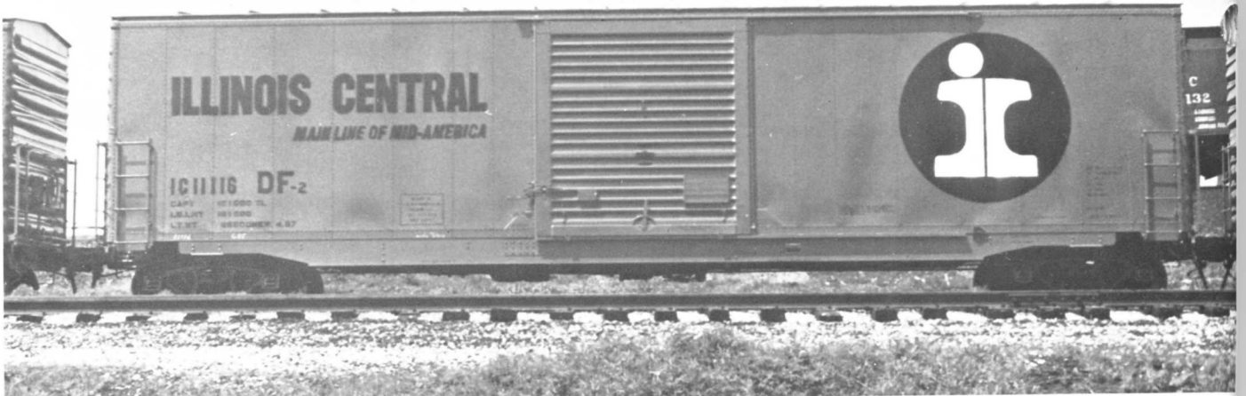
IC 11116 BOXCAR 50FT. PHOTO ICRR CENTRALIA SHOP EMPLOYEES - ICHS COLLECTION. 11000 to 11299 series cars built by the IC Centralia, IL car shop in 1967. Cars equipped with 9 belt DF-2 Evans load devices.
