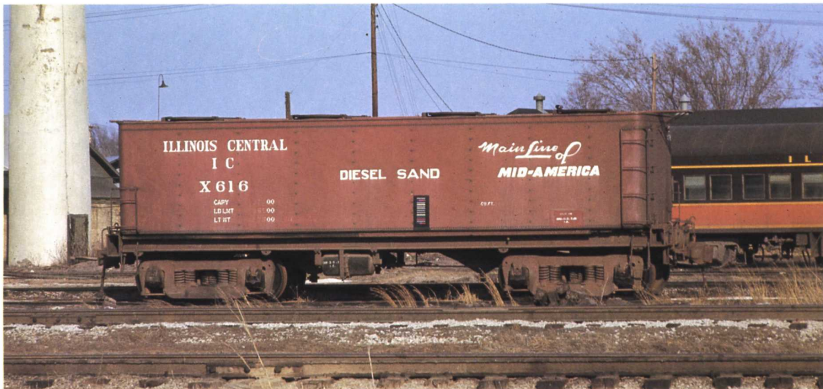
IC X616 DIESEL SAND CAR. Former A616 auxiliary tender.
