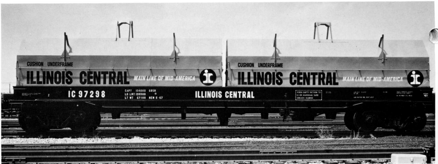
IC 97298 COIL CAR. PHOTO BY HEDRICH-BLESSING (ICRR) - ICHS COLLECTION. The 97275-97299 series cars were built in 1967 by Evans. The 100 ton capy, 48 ft. coil steel cars assigned to the Chicago area were for coil steel loading only. The cars are equipped with six movable x-members load devices.
