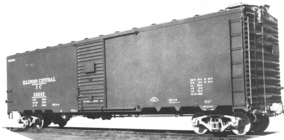
IC 33682 BOXCAR 50 FT SD. PHOTO BY ACF - ICHS COLLECTION. The 33500-33999 series cars were built by ACF in 1941 at their St. Louis, MO plant. Cars assigned to auto parts service.
