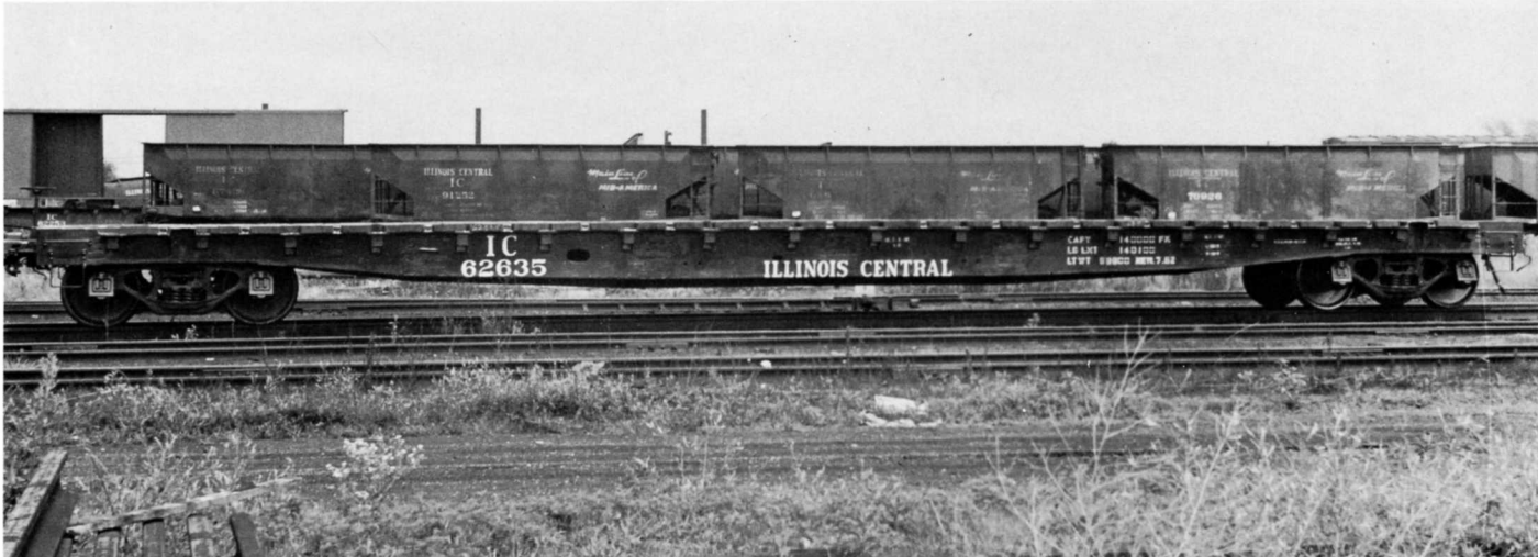
IC 62635 FLAT CAR. PHOTO BY ICRR - ICHS COLLECTION. The 62625-62674 series cars were built by the IC in 1962. The 70 ton capy cars are equipped with cast steel underframe built by General Steel Casting Co.
