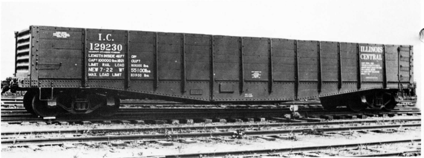
IC 129230 GONDOLA. PHOTO ACF - ICHS COLLECTION. Built by ACF in 1922 and equipped with steel drop ends and solid bottoms. Cars were renumbered to 97000-97248 series in 1940 during a rebuilding program.
