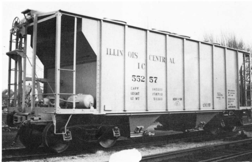
IC 55257 COVERED HOPPER PHOTO BY ACF - ICHS COLLECTION. The 55200-55299 series cars were built by ACF in 1958 with 70 ton capy. Large numbers of these cars were assigned to cement service.
