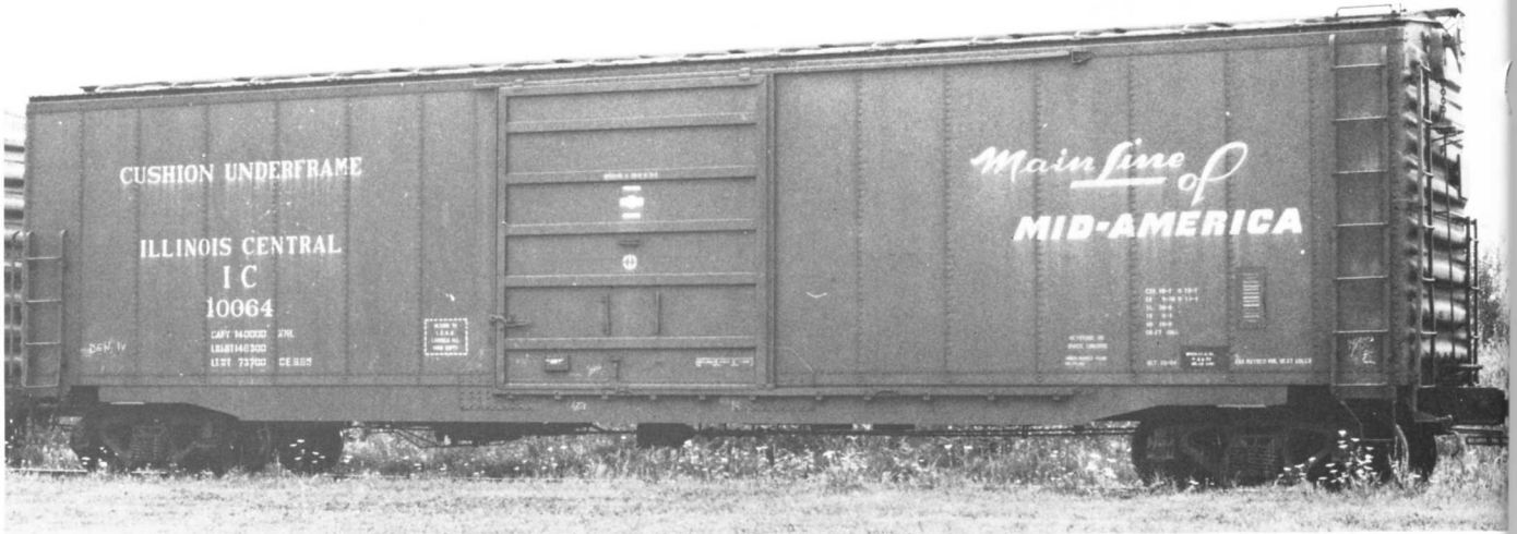
IC 10064 BOXCAR 50FT. PHOTO BY BRUCE MEYER. The 10000-10199 series cars were built by the IC Centralia, IL car shop in 1964. The cars are 70 ton capy equipped with nailable steel floors and 3 DF-2 partial belts load devices.
