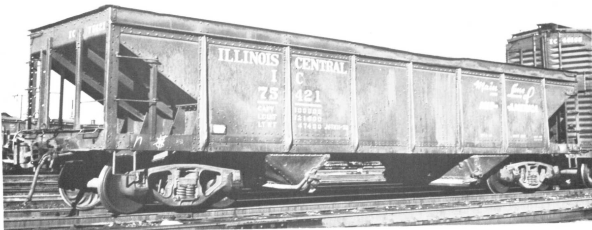
IC 75421 HOPPER. PHOTO ICRR - ICHS COLLECTION. The 75000-76999 series 50 ton copy cars were rebuilt by the IC in 1945. From former 90000-93970 hoppers built in 1921.
