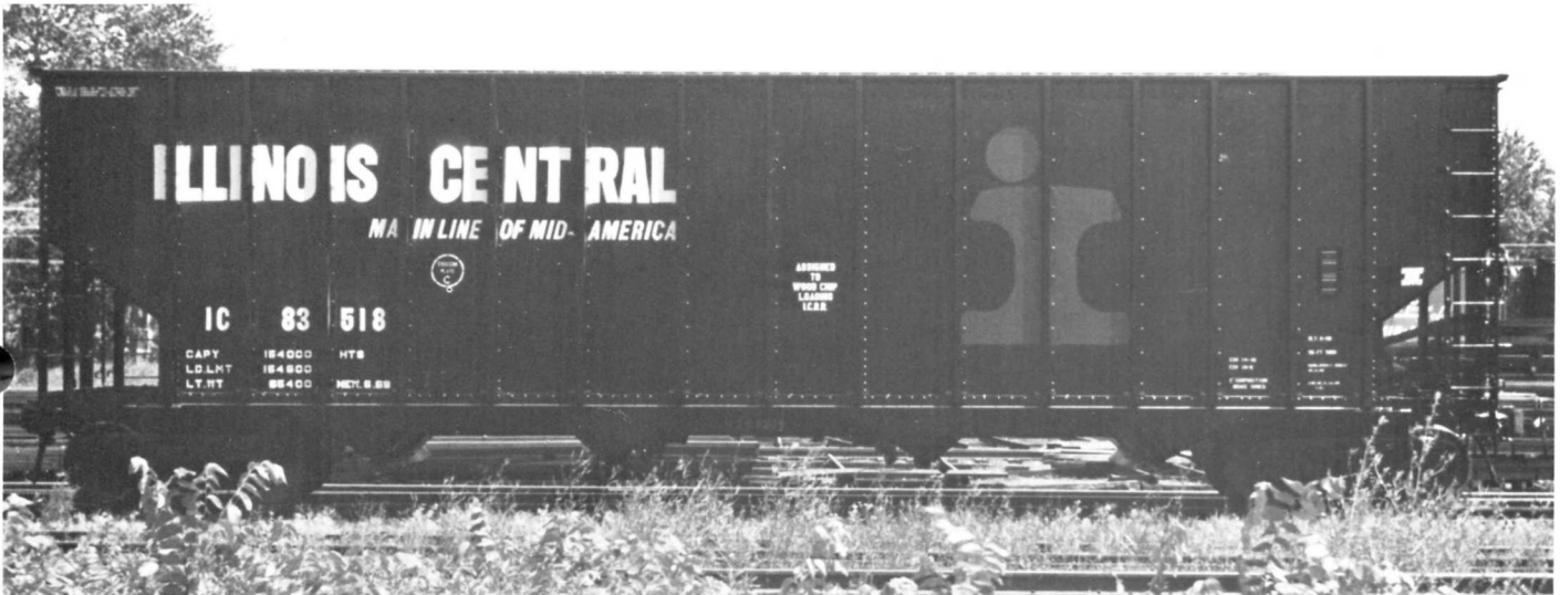
IC 83518 HOPPER. PHOTO BY ICRR - ICHS COLLECTION. The 83500-83599 series cars were built by the IC Centralia car shop in 1969. The 70 ton capy cars were assigned to wood chip loading only.
