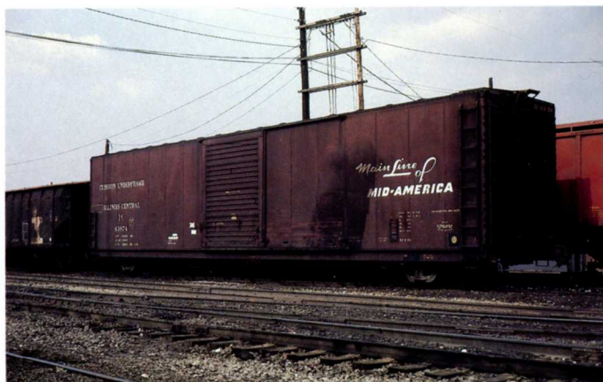
IC 43874. 60FT SD BOXCAR. 43800-43906. Thrall 1965. 70 ton capacity.
