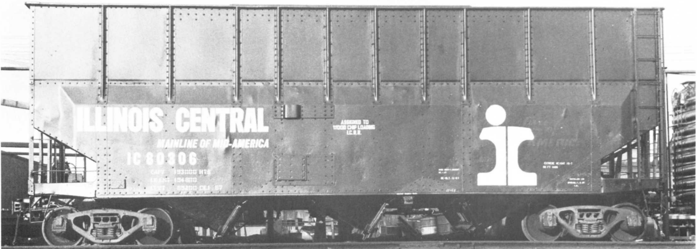
IC 80306 HOPPER. PHOTO BY ICRR - ICHS COLLECTION. The 80300-80499 series cars were built by the IC Centralia car shop in 1967. The 70 ton capy cars were assigned to wood chip loading only.
