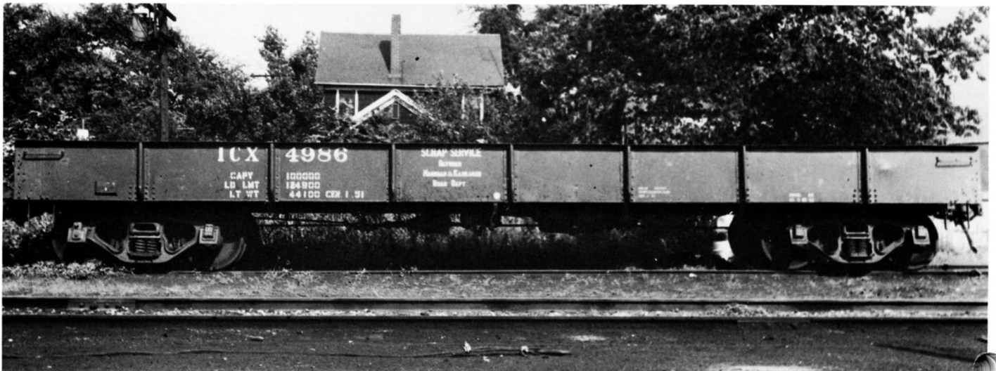
IC X4986 LOW SIDE GONDOLA. G.V. CARSON - ICHS COLLECTION. Rebuilt low side gondola assigned to scrap service for the MW depot between Markham Yard (Chicago) and Kankakee, IL.
