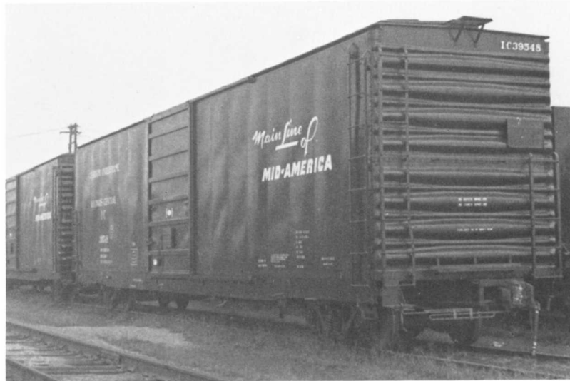
IC 39548 BOXCAR 60FT. PHOTO BY ICRR - ICHS COLLECTION. The 39536-39599 series cars were built by the IC Centralia, IL car shop in 1966. The 70 ton capy cars are specially equipped to handle Chevrolet auto parts.
