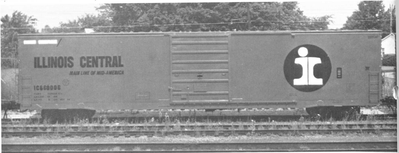
IC 660006 BOXCAR 60FT. PHOTO ICRR CENTRALIA SHOP EMPLOYEES - ICHS COLLECTION. The 660001 to 660025 series cars were built by the IC Centralia, IL car shop in 1970. Equipped with cushion underframe and 22 belt DF-1 load devices.
