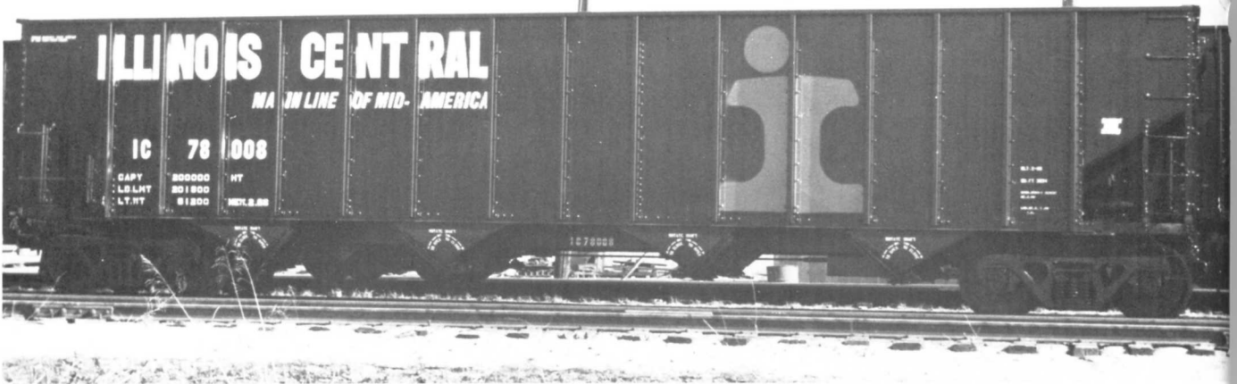
IC 78008 HOPPER. PHOTO ICRR - ICHS COLLECTION. The 78000-78999 series cars were built by the IC Centralia car shop in 1968. They were the first 100 ton capy hoppers owned by the IC.
