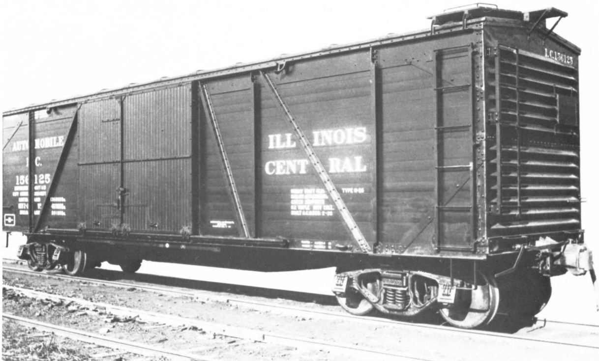
IC 156125 WOOD BOXCAR. PHOTO BY ACF - ICHS COLLECTION. The 156001-156500 series cars were built by ACF in 1925 at their Madison plant in Chicago area. Renumbered by the IC later to 11000 to 11974 series. Assigned to automobile service.
