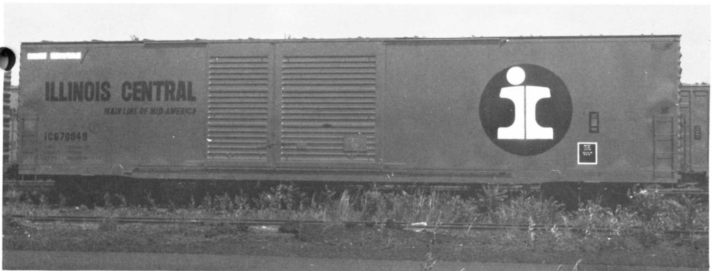
IC 670049 BOXCAR 60FT. PHOTO IC CENTRALIA SHOP EMPLOYEES - ICHS COLLECTION. This car is part of the 670036 to 670075 series built by the IC Centralia, IL car shop in 1972. Assigned to auto parts service.
