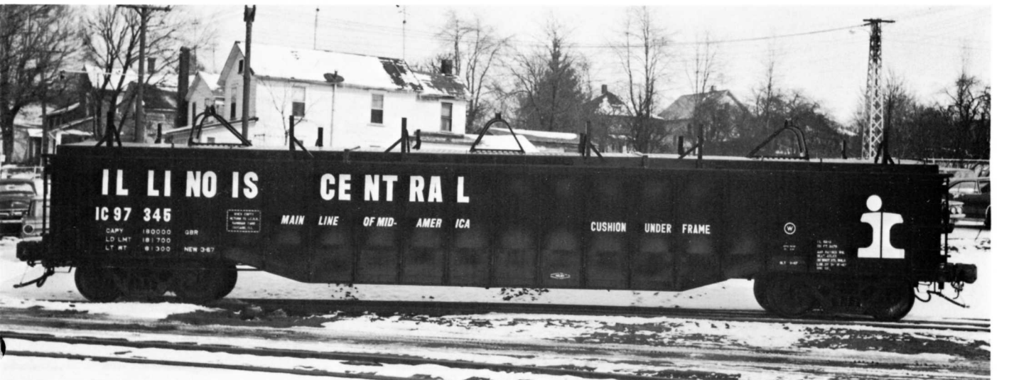
IC 97345 COVERED GONDOLA. PHOTO BY ICRR - ICHS COLLECTION. The 97300-97349 series covered gondolas were built by Greenville in 1967 for steel service in Chicago area. The cars are of 100 ton capy and are equipped with a three section removable roof.
