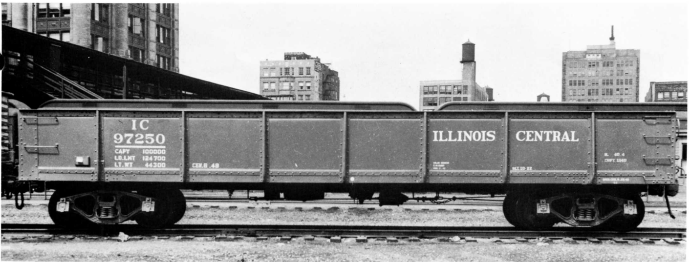
IC 97250 LOW SIDE GONDOLA. PHOTO BY ICRR - ICHS COLLECTION. 97250-97251 were 70 ton, 41 ft solid bottom gondolas converted by the IC Centralia car shop in 1950 from 203700-205839 series gondolas built in 1923. 97250 & 97251 were rebuilt for carrying LCL containers for lime & cement. The cars were equipped to carry 10 containers of 145 cuft capy per car.
