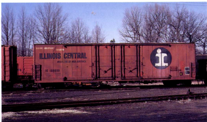
IC 150059. 50 FT. DD BOXCAR. 150025-150079. USRE 1972. 70 ton capacity.
