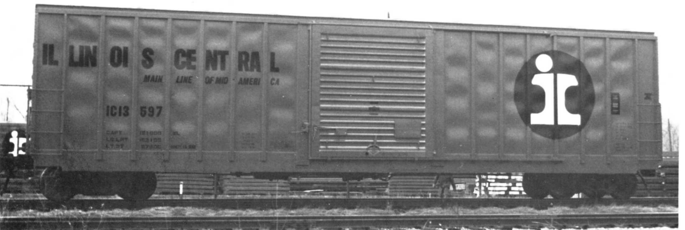
IC 13597 BOXCAR 50 FT. PHOTO IC CENTRALIA SHOP EMPLOYEES - ICHS COLLECTION. 13400 to 13599 series cars built by the IC Centralia, IL car shop in 1969. Cars equipped with Belt DF-2 load devices and equipped with nailable steel floors.
