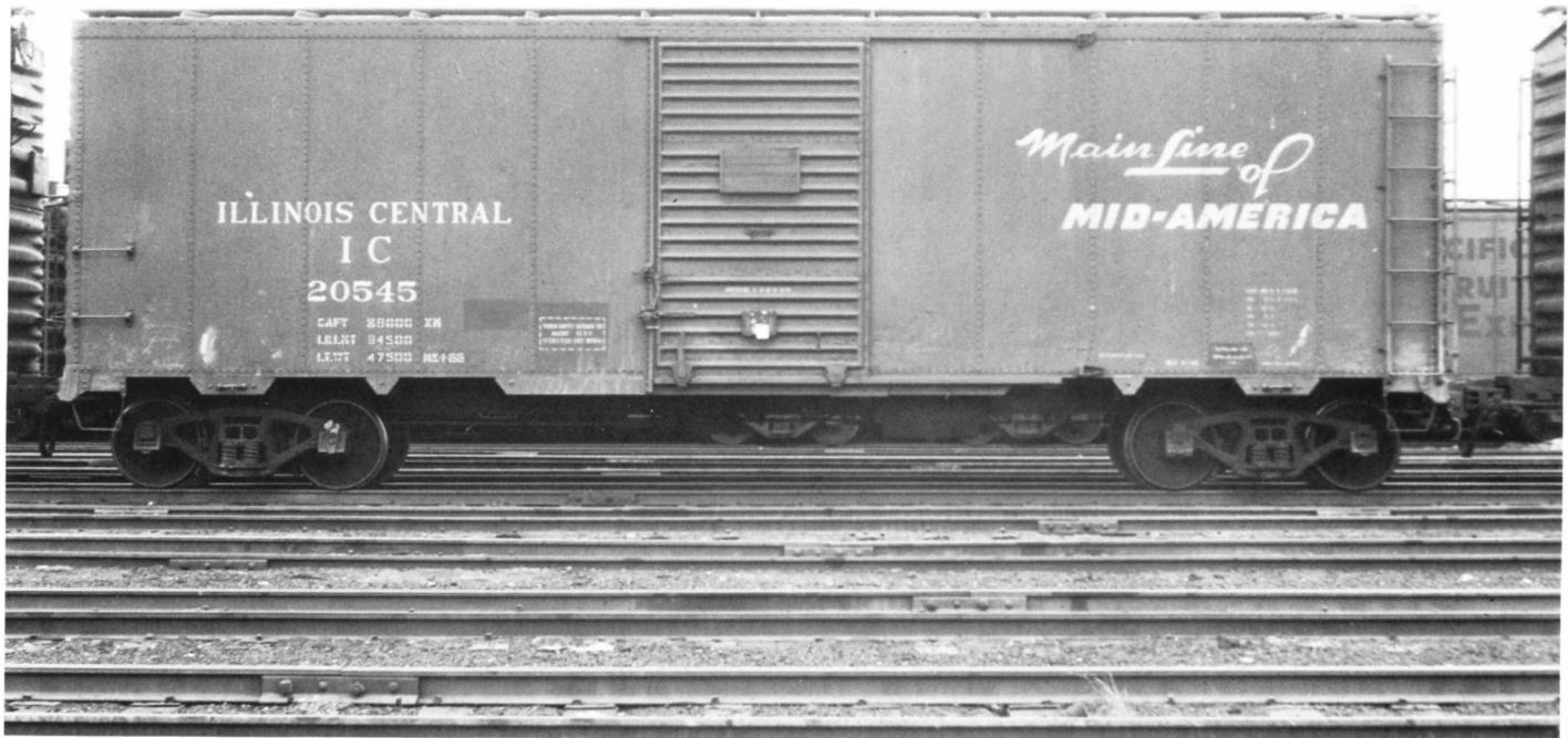
IC 20545 BOXCAR 40FT. PHOTO BY W.C. THURMAN - DAVID J. DAISY COLLECTION. The 20000-20999 series cars were built by Pullman Standard - Bessemer plant in 1940. Cars were upgraded by the IC McComb, MS car shop in 1966. This is one of 15 cars equipped with 5 belt DF loading devices for special loading.
