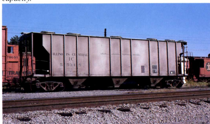
IC 55345. COVERED HOPPER. 55300-55499. Pullman Standard 1965. 70 ton capacity.
